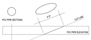
LOCATE CUT LINE BY MEASURING APPROX . LENGTH OF OVAL ALONG PIPE ELEVATION ALL OVALS LINERS ACHIEVED WITH 12" OR 18" NO. STANDARD PVC PIPING
